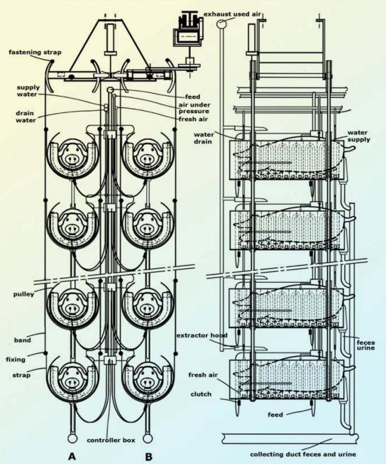
To prevent large air movements in the barn, the pigs are cooled or heated with water in a closed-loop system. In the summer day the heated cooling water is stored to be used again in the winter to heat the pigs. Fresh air at the head of the animal is collected again, together with the exhaled air, by an extractor hood, after which this air is purified and made ready for use, after which it is offered again at the head of the animal.
